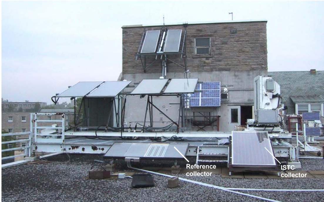
Figure 6: Outdoor test setup used to evaluate the ISTC solar collector.
