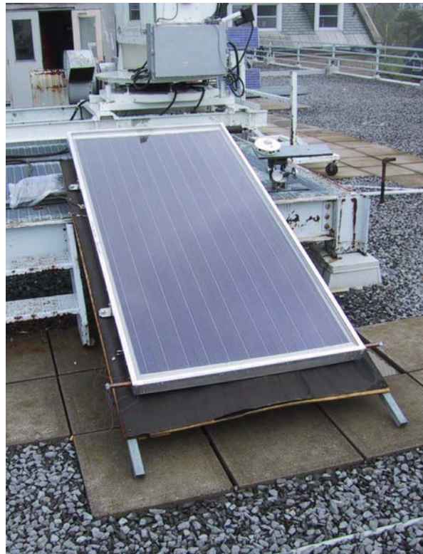
Figure 3: Prototype solar collector with the Integral Stagnation Temperature Control (ISTC) feature constructed for this study.
