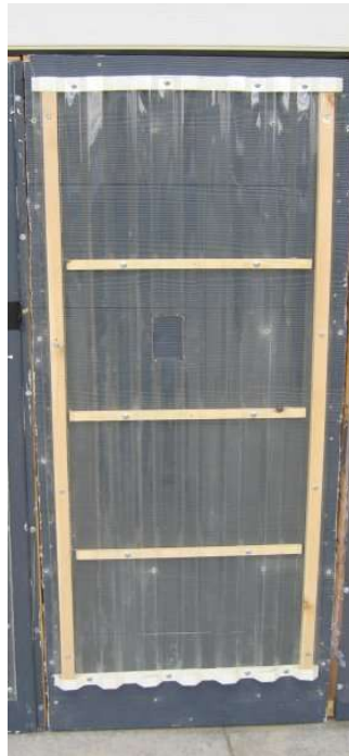
Illustration 1 Low Tech Collector -- Test Panel
